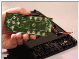
• Once unscrewed. gently pull upwards detaching the button panel from the casing.
