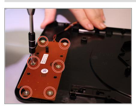
On the bottom side of the disk flap case, the back of the button panel will be visible. Using a Philips J0 screwdriver, unscrew all 6 screws.
