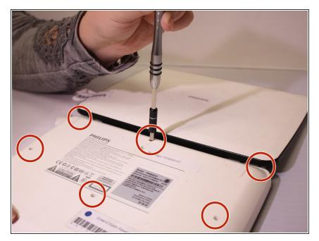
Lay the player flat so the outside casing is facing upwards. Using the screwdriver, unscrew all the case screws on the bottom of the player.
